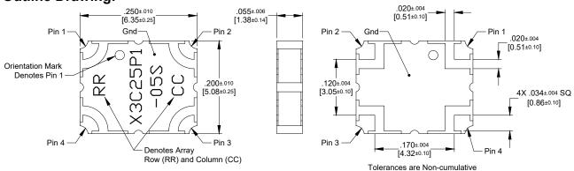
Dimensions are in Inches [Millimeters] X3C25P1-05S Mechanical Outline
