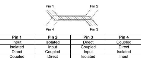
\*Notes: The direct port has a DC connection to the input port and the coupled port has a DC connection to the isolated port.
