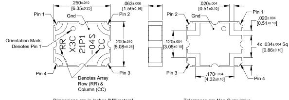
Dimensions are in Inches [Millimeters] X3C21P1-04S Mechanical Outline
