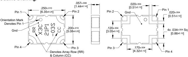
Dimensions are in Inches [Millimeters] X3C21P1-03SS Mechanical Outline
