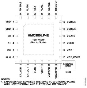
Figure 2. Pin Configuration
