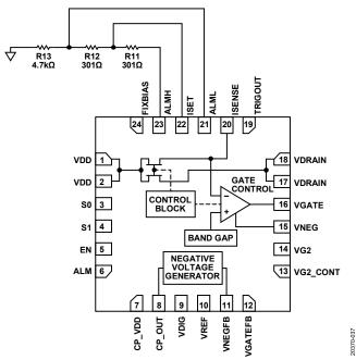
Figure 37. Current Alarm Resistor Configuration for  $\pm 6\%$  Thresholds
