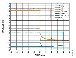
Figure 24. Shutdown Waveform (Negative Voltage Generator Used and EN Controlled, HMC637ALP5E Used as External Amplifier)
