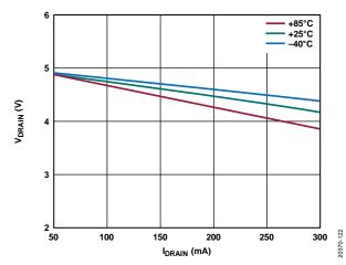
Figure 22. V<sub>DRAIN</sub> vs. I<sub>DRAIN</sub> Across Temperature, VDD = 5 V, VDIG = 3.3 V, S0 = Ground, S1 = Ground
