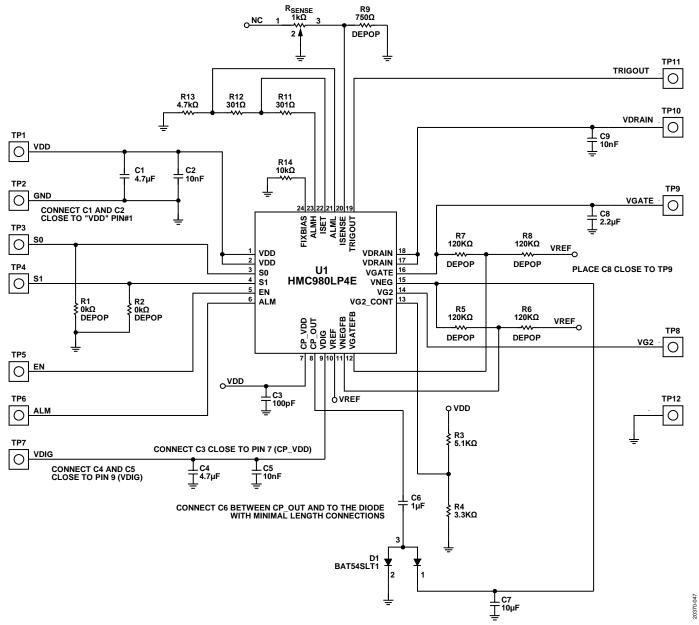
Figure 47. Evaluation Board Schematic
