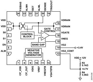
Figure 36. Resistor Divider Used to Set VG2
