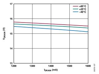
Figure 25. V<sub>DRAIN</sub> vs. I<sub>DRAIN</sub> Across Temperature, VDD = 16.5 V, VDIG = 5.0 V, S0 = VDIG, S1 = VDIG
