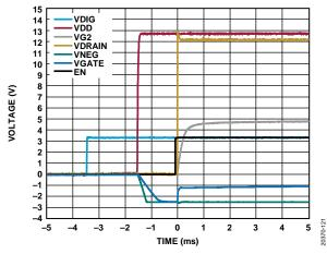
Figure 21. Power-Up Waveform (Negative Voltage Generator Used and EN Controlled, HMC637ALP5E Used as External Amplifier)
