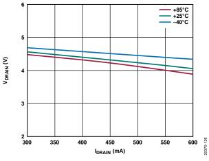
Figure 26. V<sub>DRAIN</sub> vs. I<sub>DRAIN</sub> Across Temperature, VDD = 5 V, VDIG = 3.3 V, S0 = 3.3 V, S1 = Ground
