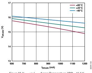
Figure 23. V<sub>DRAIN</sub> vs. I<sub>DRAIN</sub> Across Temperature, VDD = 16.5 V, VDIG = 5.0 V, S0 = Ground, S1 = VDIG
