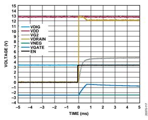
Figure 17. Enable Waveform (Negative Voltage Generator Used, HMC637ALP5E Used as External Amplifier)
