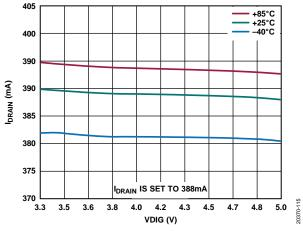
Figure 15. I<sub>DRAIN</sub> vs. VDIG, HMC637ALP5E</sub> Used as External Amplifier, S0 = VDIG, S1 = Ground
