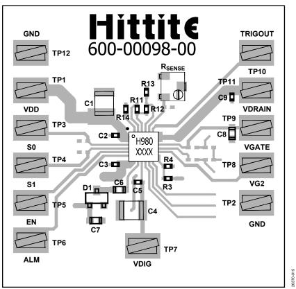
Figure 48. Evaluation Board Component Side Layout
