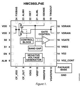
The HMC980LP4E allows stable RF amplifier biasing over supply, temperature, and process variations, and eliminates the required calibration procedures usually employed to prevent RF performance degradation due to variations in amplifier drain current.
