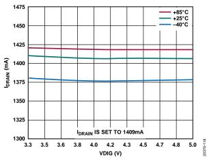
Figure 18.  $I_{DRAIN}$  vs. VDIG, HMC637ALP5E Used as External Amplifier, S0 = VDIG, S1 = VDIG
