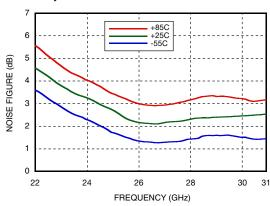
Noise Figure vs. Temperature @ Vdd = +5V
