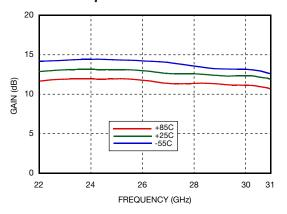
Gain vs. Temperature @ Vdd = +5V
