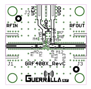
**GRF400X Evaluation Board Assembly Diagram**
