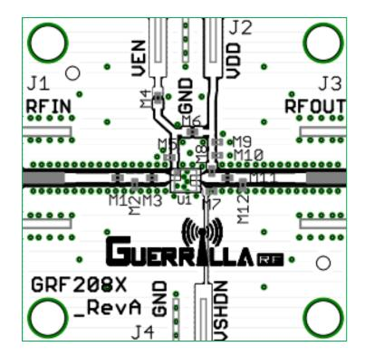
**GRF2081 Evaluation Board Assembly Diagram**
