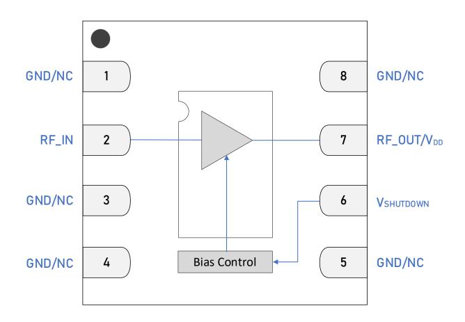
2.0 x 2.0 mm DFN-8 Pin Out (Top View)
