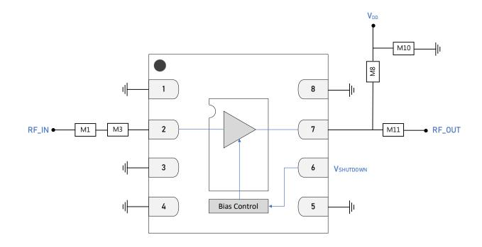
**GRF2081 Standard Test Schematic**
