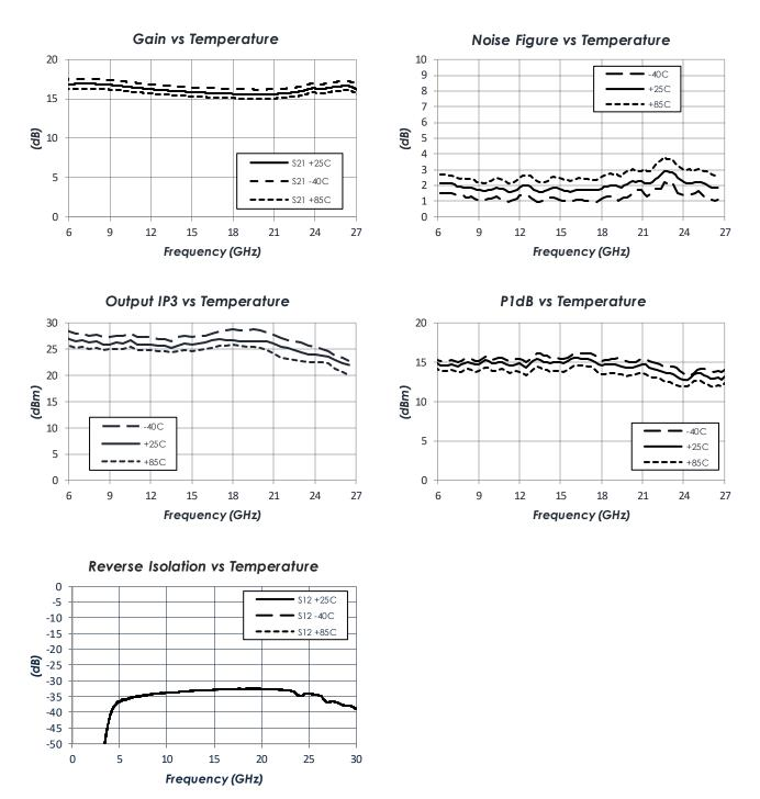
OIP3 Test Conditions: Two -15dBm tones at input with 10 MHz spacing.
